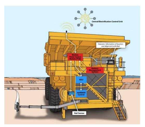
Central electrification control unit and on vehicle architecture
