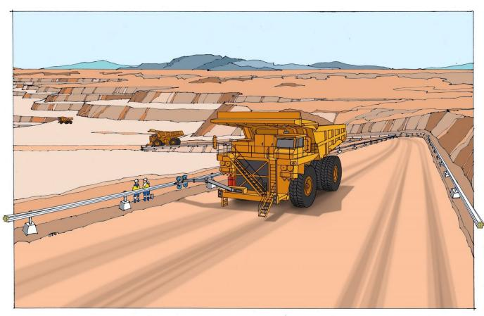
BluVein safe slotted rail installed near to ground for easier, lower cost installation and operation.
